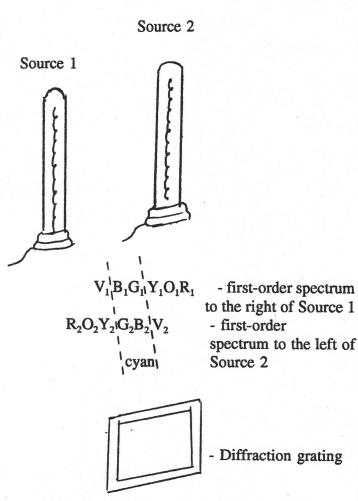
At an appropriate distance from the two bulbs, the observer can see two first-order spectra overlapping. The appropriate distance between the bulbs and the observer depends on the separation of the bulbs and the number of lines per millimetre on the diffraction grating.
